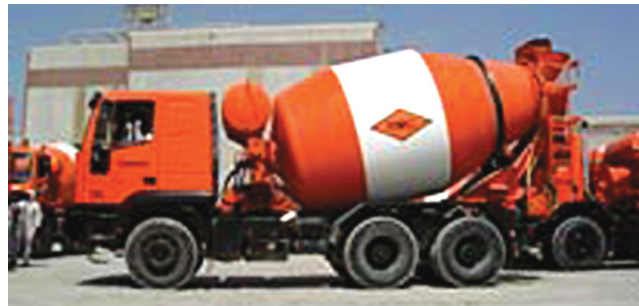
Truck used for carrying premixed concrete
