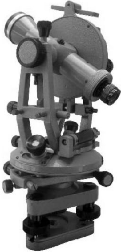
Photo Transit Vernier Theodolite 20"
